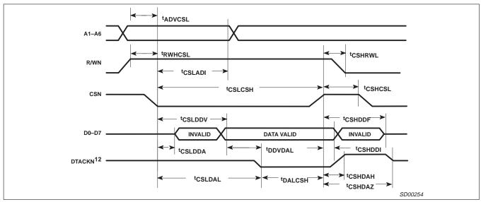
Figure 2. Read Cycle Bus Timing
