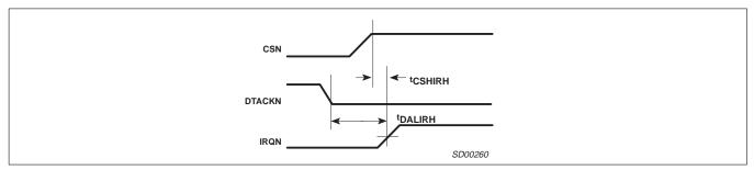
Figure 8. Interrupt Timing, Write Cycle
