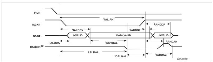
Figure 4. Interrupt Cycle Timing
