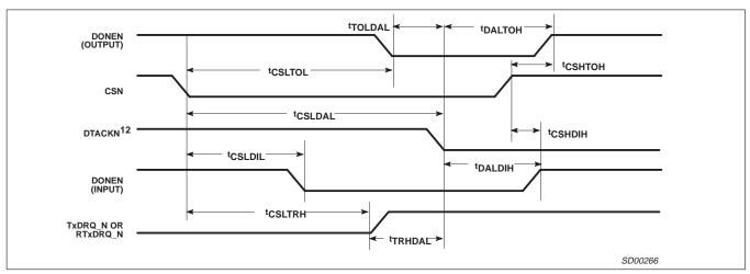
Figure 14. Transmit, Dual Address DMA
