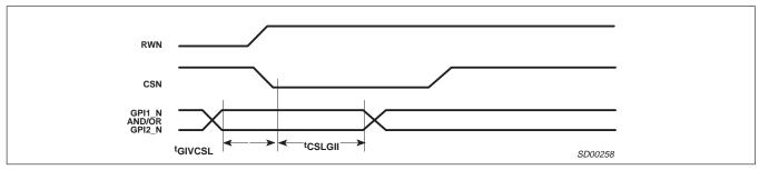
Figure 6. Input Port Timing
