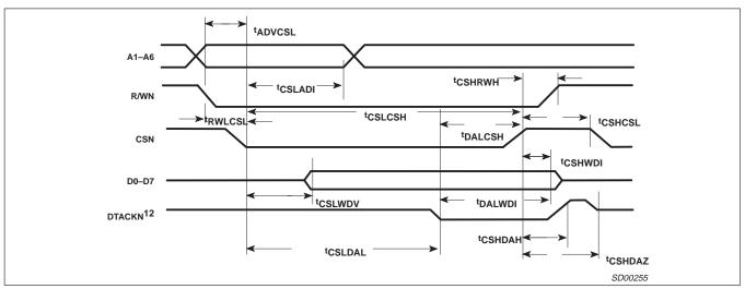
Figure 3. Write Cycle Bus Timing
