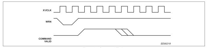
Figure 19. Command Timing
