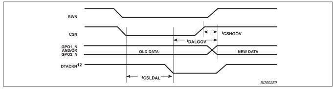
Figure 7. Output Port Timing
