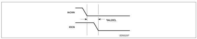
Figure 5. Interrupt Daisy Chain Timing
