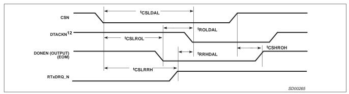
Figure 13. Receive, Dual Address DMA
